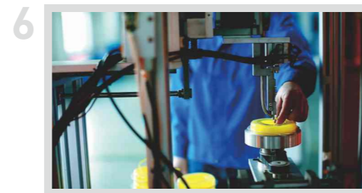
6 Winding: Auto machine to ensure the length
